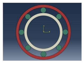
The geometry is simple. The bearing has an inner ring diameter of 30 mm, the outer ring diameter of 45 mm. There are eight cylindrical rollers with a diameter of 5mm. No friction is assumed in the model.
